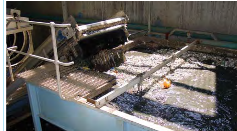
The Arrowbio plant in Tel Aviv, Israel, uses flotation to sort the waste.
